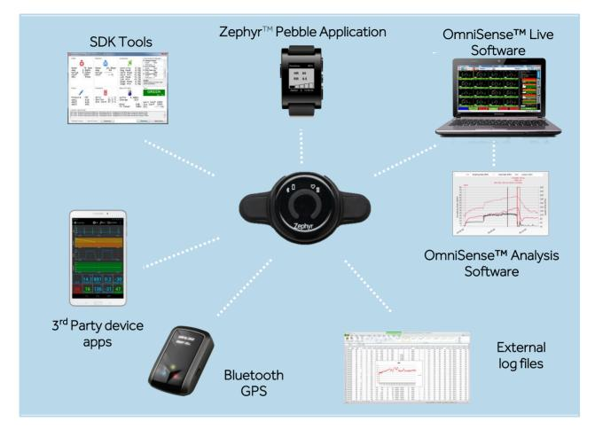
The BioPatch<sup>™</sup> HP monitoring device can transmit live physiological data, or download log data to a variety of platforms:
