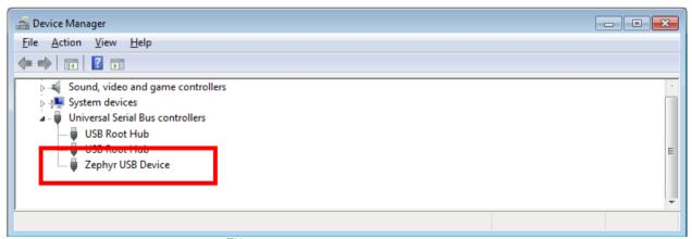
When installed, the BioModule<sup>TM</sup> will display in Windows® Device Manager as a *Zephyr USB Device*.
